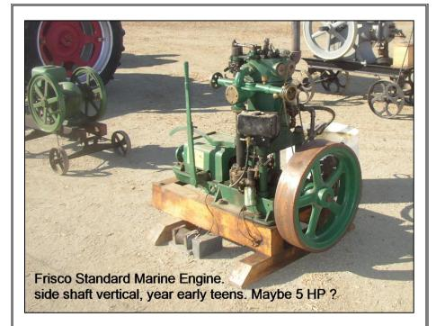
An engine that is a real crowd pleaser, is Carl Ross's marine engine from a boat. It gets its cooling from the river the boat sits in, and for display purposes Carl uses a wash tub. The boat engine runs on gasoline.
