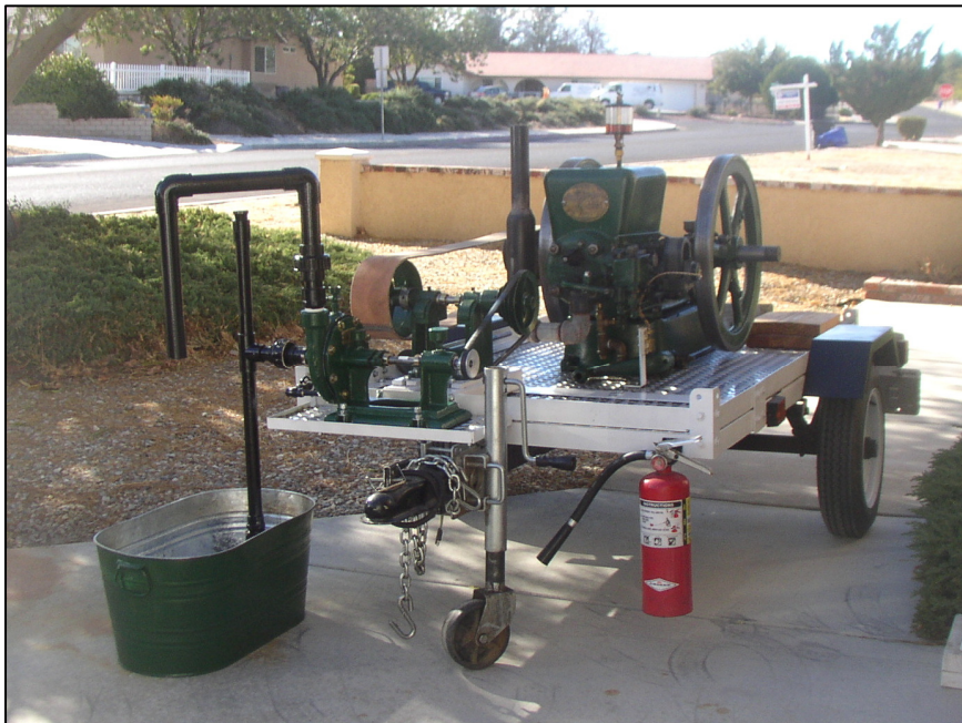
Pictured above, is Ron & Bob's 1917 Fairbanks Morse 3 hp throttler, flat belted to a 1940's antique centrifugal water pump.
