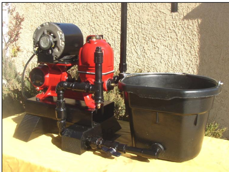
Pictured above is a 1950'S "Dayton" Double Action, Piston, Shallow Well Water Pump. Manufactured by "F.E. Meyers & Bros" out of Ashland, Ohio, for "Dayton". Rebuilding was done last fall by editor, Bob Hanson.
