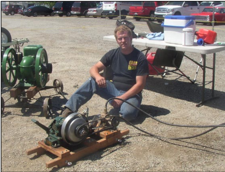
Zackary Forbes brought his 1930's Maytag Model 92 Engine, driving a water Pump Nozzle Display.
