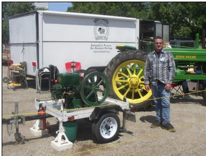
On the trailer, Ron & Bob Hanson's 1917 Fairbanks Morse, Throttling Governor, 3 HP "Z" Series, Ignitor Model, with a Splitdorf Magneto.
