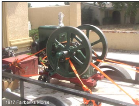
Still sitting on the trailer, is Bob & Ron Hanson's 1917 Fairbanks Morse, Throttling Governor, 3 HP "Z" Series, Ignitor Model, with a Splitdorf Magneto. Rare Find..... Hope to have it running for Mojave Trail Days, in Oct.
