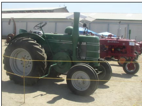
Pictured left is Carl’s new 1949 Field Marshall Tractor, better known as the Shot Gun Engine. 40 HP, 2 Cycle Diesel Monster, weighing 7000 lbs.
