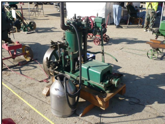
Carl Ross brought a 5 HP, Frisco Standard Marine Engine. Made in California. Very interesting, with a gear box for reversing.
