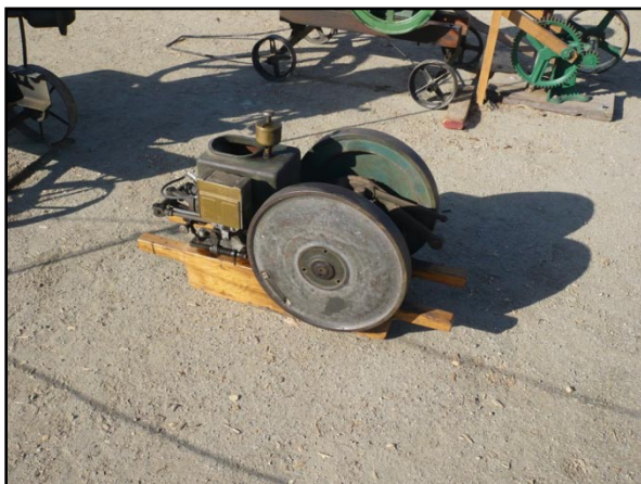
Carl Ross brought an interesting engine to the show. 1 1/2 HP ALPHA, De- Laval Separator Engine.
