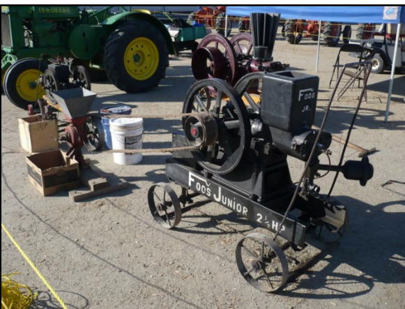
Carl's 1917, 2 ½ HP Foos Junior engine belted to a corn grinder, with a corn Sheller in the back ground.
