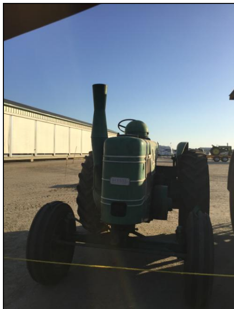
Pictured left is Carl's 1949 Field Marshall Tractor, better known as the Shot Gun Engine. 40 HP, 2 Cycle Diesel Tractor. Carl has to load and fire a 12 ga. shot gun shell, to get this tractor started. And is it loud when you forget to close the front cylinder head plug.....
