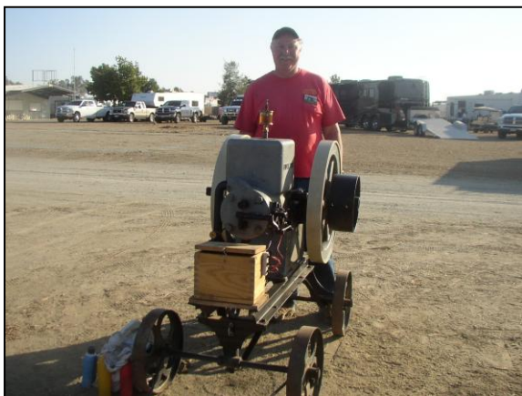
1 1/2 HP John Deere hit & miss with a Maytag driving a grinding wheel.
