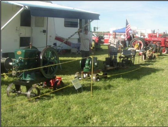
Bob Hemphill is standing next to his trailer and displaying his 6 HP, 1922 Fairbanks Morse, Model "Z" Engine, pictured left.
