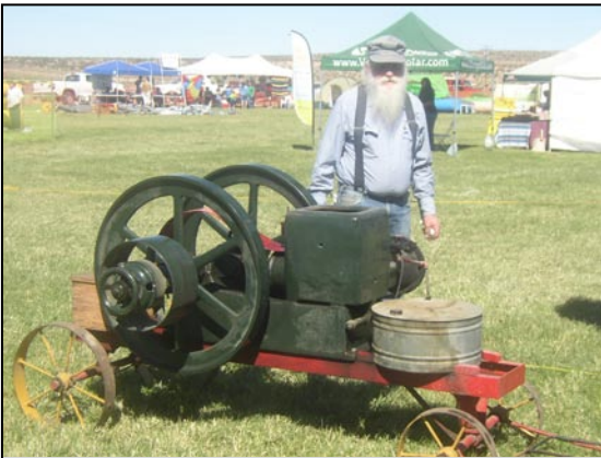
A nice picture of Carl Ross standing next to his large 1917, Witte 6 HP Head less engine. Great running engine.
