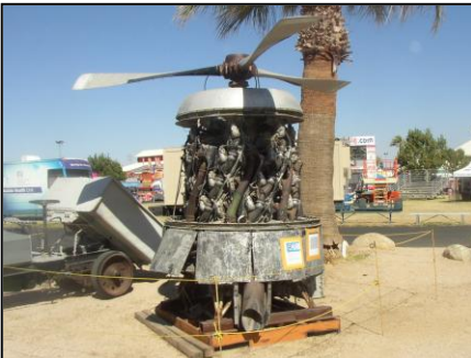
Another one of Paul Ogden's specials. Pratt & Whitney R-4360, 28 cylinder Radial Wasp Piston Airplane Engine. Displacement 4,362 cu in.
