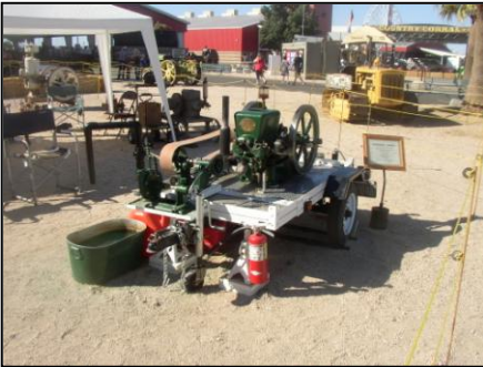
Pictured left is Bob Hanson's 1917, 3 HP Fairbanks Morse, throttler engine, pumping green water. We call "Gatorade"...
