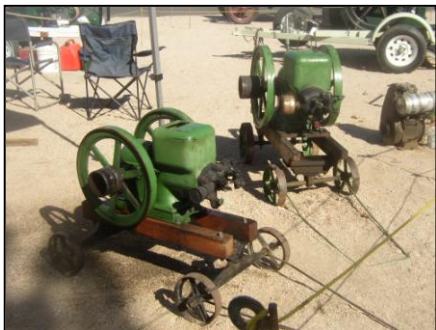
Pictured left are two John Deere hit & miss engines, brought in by Bill Forbes. The first one is a 1931, 1 1/2 HP and the larger one is a 3 HP, 1921 John Deere
