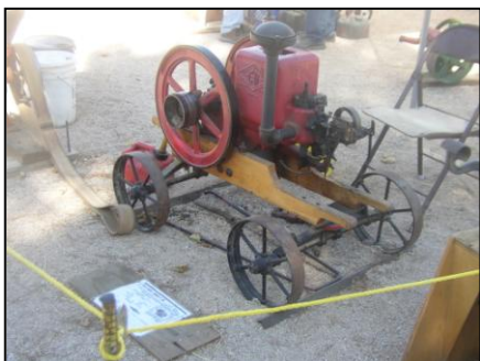
Pictured left is Carl Ross's 1918, 1 1/2 HP, Emerson Brandingham Engine, belted to a C.S. Bell Company Grinder, from the late 1800's.
