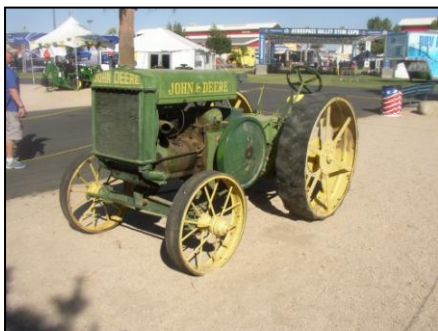
Pictured left is the clubs 1925, two cylinder, John Deere, Model "D" Tractor. It Runs great & makes a lot of noise.....
