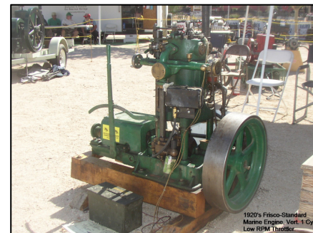
Pictured left is a 1920's Marine Engine, Manuf. By Frisco Standard. Vert. 1 cye. Low rpm, water cooled. Owner Carl Ross
