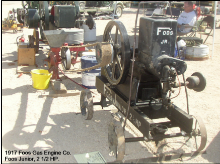
Pictured left is a 1917, 2 1/2 HP Foos Gas Engine Co. Foos Junior, belt driving a corn grinder. Owner Carl Ross.
